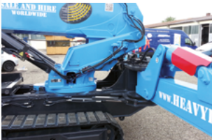
Hydraulic fold-out support
