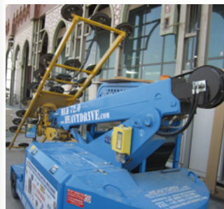
The industrial crane MLK 72.0 with 4-axis manipulator, which set the triangular and trapezium-shaped glass panes of up to 1,800 kg.
