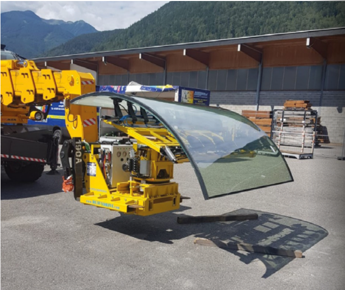
Extremely low overhead suction point of 1m above the floor
